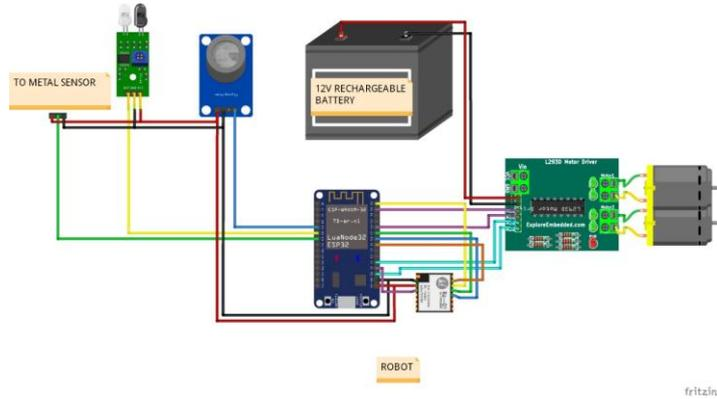
Fig -4: Descriptive Diagram of Robot
