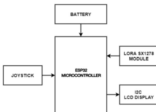
Fig -2: Block Diagram of Remote-control
