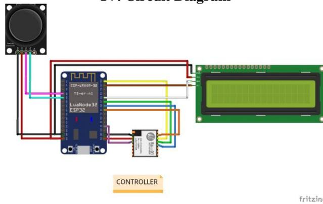
Fig -3: Descriptive Diagram of Remote Control
