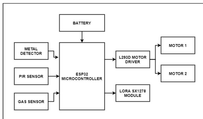
Fig -1: Block Diagram of Robot
